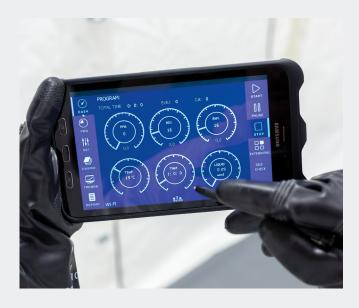
Sophisticated Cleamix control software enables hydrogen peroxide- and water vapor levels to be maintained below saturation point and risk of H<sub>2</sub>O<sub>2</sub> condensation accumulating on surfaces is minimized.
