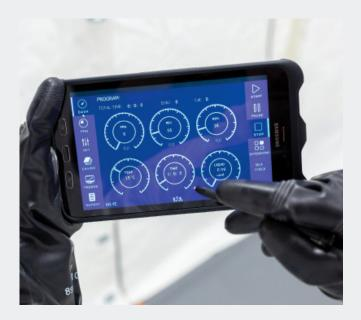
Sophisticated Cleamix control software enables hydrogen peroxide- and water vapor levels to be maintained below saturation point and risk of  $H_2O_2$  condensation accumulating on surfaces is minimized.
